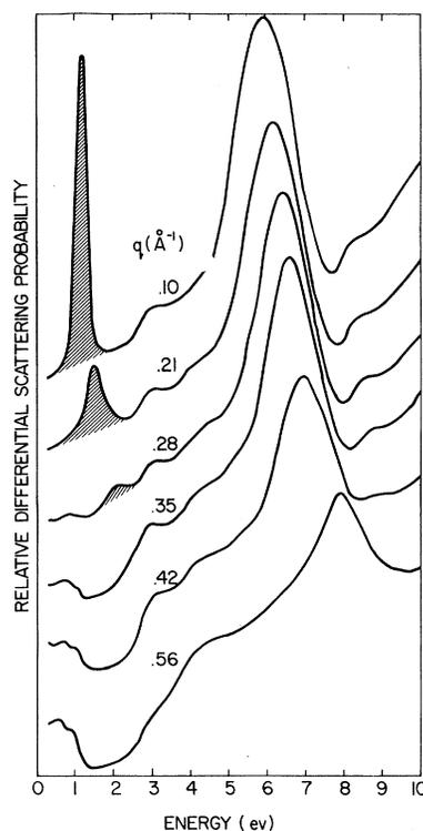
FIG. 1. Momentum dependence of electron energy-loss probability measured in stage-1  $\text{FeCl}_3$ -intercalated graphite.  $\vec{q}$  parallel to graphite planes.
