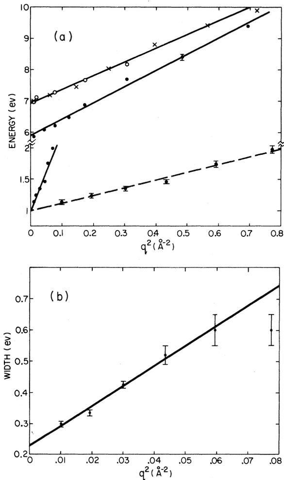
FIG. 2. (a) Plasmon dispersion: solid dots, intercalated graphite; open circles, HOPG; crosses, crystalline graphite (Ref. 4); the dashed line is through 1-eV plasmon data redrawn on 10 $\times$  expanded scale. (b) FWHM of 1-eV plasmon.
