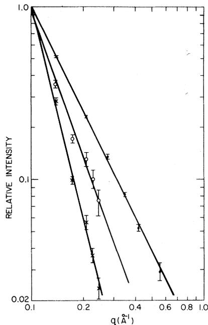
FIG. 3. Momentum dependence of plasmon intensity: solid circles, 5.9-eV plasmon peak height  $\propto q^{-2.06}$ ; crosses, 1-eV plasmon peak height  $\propto q^{-4.1}$ ; open circles, 1-eV plasmon integrated strength  $\propto q^{-2.8}$ .
