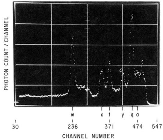
FIG. 2. Satellite line spectrum of the heliumlike iron (Fe XXV) in PLT as recorded by a multichannel analyzer. The photon energy decreases with increasing channel number. The conversion gain is 0.18 eV/channel. *w* indicates the Fe XXV  $K\alpha$  resonance line at 1.85 Å used for Doppler-broadening measurements.
