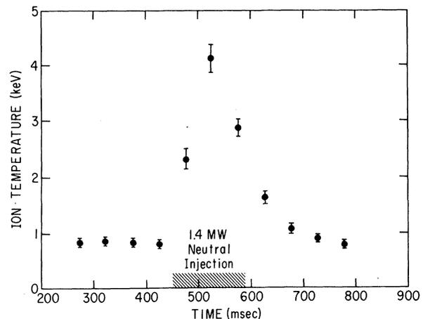
FIG. 4. Ion temperature derived from Doppler broadening of the Fe XXV  $K\alpha$  line at 1.85 Å. Each point is taken over an integration time of 50 msec.
