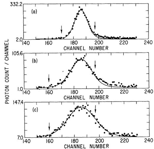
FIG. 3. Line profiles of the Fe XXV  $1s^2(1S)-1s2p(1P^0)$  resonance transition obtained during time intervals of 50 msec (a) before and (b), (c) during neutral-beam injection. The conversion gain is 0.18 eV/channel. In order to determine the ion temperature, Voigt functions are fitted to the data. Shown are the curve fits for the times (a) 0.425, (b) 0.475, and (c) 0.525 sec of Fig. 4.
