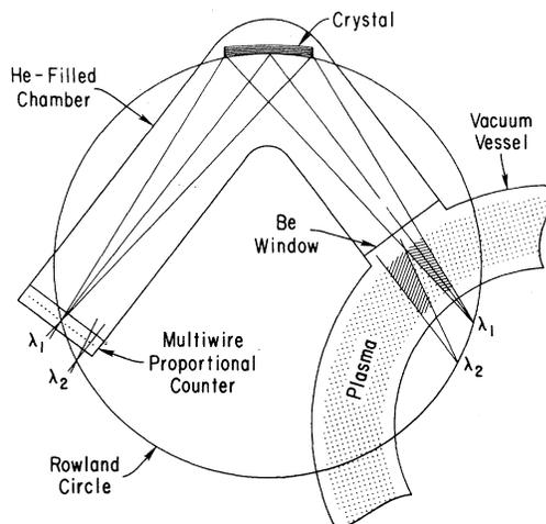
FIG. 1. Quartz-crystal spectrometer in the Johann configuration. X rays emitted from the shaded area of the plasma pass through a beryllium window into a helium-filled tube and are Bragg reflected by the crystal onto the position-sensitive detector. Photons of different energies are focused to different detector points.
