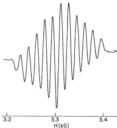
FIG. 1. Derivative of the EPR absorption spectrum from a color center in the conduction plane of  $\beta$ -Al<sub>2</sub>O<sub>3</sub>:Na as measured at 77 K and 9.3 Ghz, with  $\vec{B}$  parallel to the  $c$  axis.
