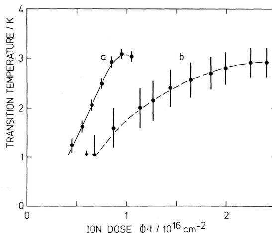
FIG. 1. Transition temperature of Pd films vs dose  $\Phi t$  of irradiating  $\text{He}^+$  ions at 130 keV. (a) 400- $\text{\AA}$  Pd condensed at 4.2 K; (b) 200- $\text{\AA}$  Pd condensed at 200 K and annealed to 300 K.
