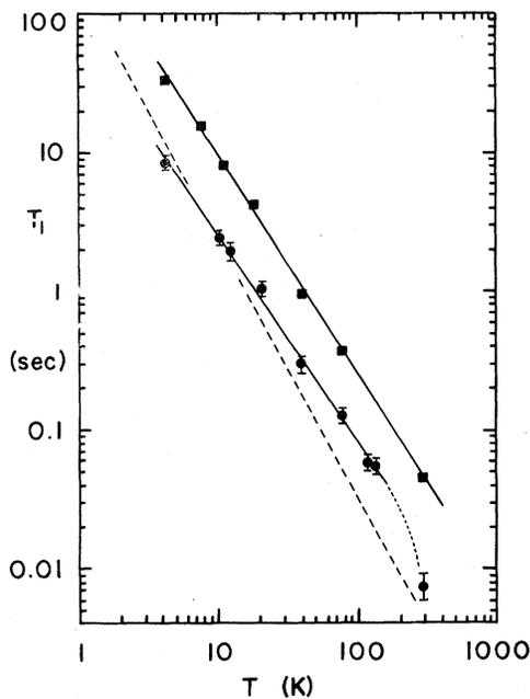
FIG. 1. Temperature dependence of  $^{75}As$  NQR spin-lattice relaxation times,  $T_1$ , in amorphous As (circles), rhombohedral As (squares), and amorphous  $As_2Se_3$  (dashed line). Solid straight lines are least-squares fits to the data.
