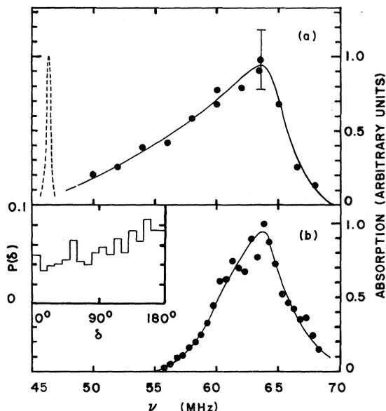
FIG. 2. (a) NQR absorption in amorphous As (circles and solid line) and rhombohedral As (dashed line) at 4.2 K. (b) Contribution to NQR line shape from bonding electrons and nearest-neighbor atoms as described in text. Inset, dihedral angle distribution from Ref. 4. The points refer to the calculated points of a histogram, while the solid line is to aid the reader's eye.
