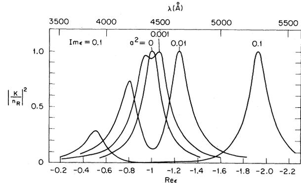
FIG. 2. The response function  $|K/n_R|^2 = |(\epsilon + 1) - [(\epsilon - 1)^2 a^2 / (\epsilon + 1)]|^{-2}$  for surface plasmons on a rough surface ( $a > 0$ ). The response function for a smooth surface is given by the curve labeled  $a^2 = 0$ . Each curve is scaled so that the maximum value of  $|K/n_R|^2$  is equal to 1.
