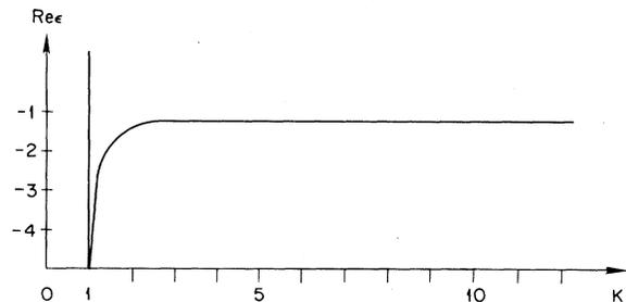
FIG. 1. Dispersion relation of surface plasma waves on a smooth surface.
