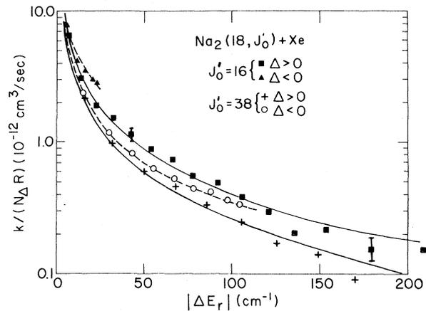
FIG. 2. Plot of  $k/N_{\Delta}R$  vs  $|\Delta E_r|$ . This is equivalent to a surprisal plot assuming the most common prior rate and would be a straight line if the exponential gap law held. Solid lines are fits for  $\Delta > 0$  points and dashed lines for  $\Delta < 0$  using power law [Eq. (5)].
