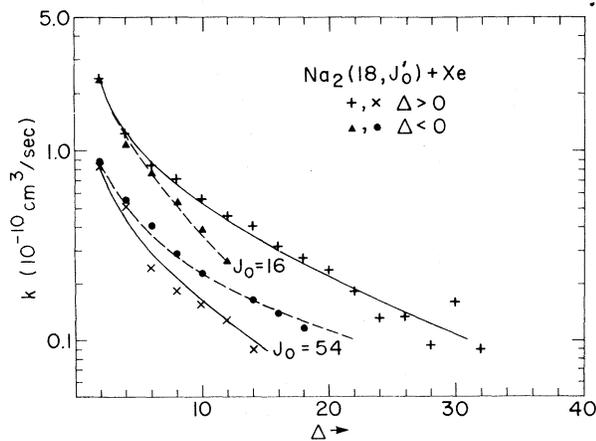
FIG. 1. Plot of measured rate constants vs  $\Delta$ . The solid lines are fitted to the  $|\Delta| > 0$  points and the dashed lines are fitted to the  $\Delta < 0$  points; both fits used Eq. (5).
