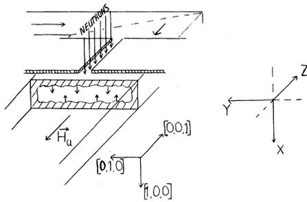
FIG. 1. Schematic view of a part of the picture frame crystal with neutron diaphragm. The coordinate system, crystal orientation, and direction of the applied field and magnetization are indicated. The arrows in the cross section indicate how the wavy-structured domain walls move towards the center of the specimen (sandwich model).
