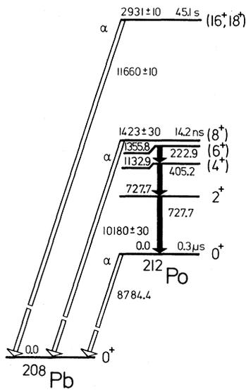
FIG. 2. Partial level scheme of  $^{212}\text{Po}$ .
