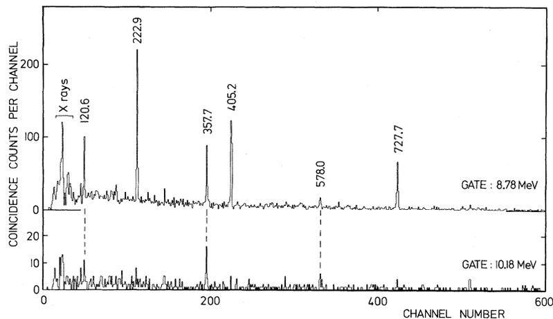
FIG. 1. Coincidence spectra gated on the 9.78- and 10.18-MeV  $\alpha$  lines of  $^{212}\text{Po}$ .
