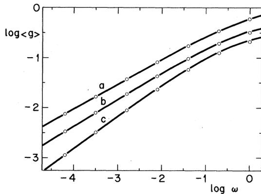
FIG. 2.  $\langle g \rangle$ , the average value of  $g$  [Eq. (3)] for three different distributions of  $W$ 's: (a)  $W$  uniformly distributed in  $\frac{1}{2} \leq W \leq \frac{3}{2}$ ; (b)  $W$  uniformly distributed in  $0 \leq W \leq 1$ ; (c)  $\rho(W) = \frac{1}{2}W^{-1/2}$  for  $0 \leq W \leq 1$ . Monte Carlo results (circles) are compared with the predictions  $g_0 \approx \langle g \rangle$  of Eq. (9) (full curves).
