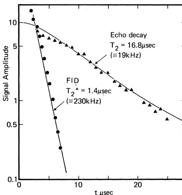
FIG. 3. FID and echo decay for the 16.7-MHz transition of  $\text{LaF}_3:\text{Pr}^{3+}$  at 2.0 K. For the echo, the solid line is calculated using Eq. (5.7) of Ref. 15.
