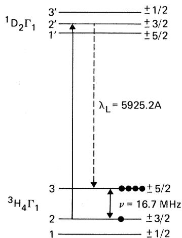
FIG. 1. Energy level diagram for the 5925.2-Å transition of LaF<sub>3</sub>:Pr<sup>3+</sup> showing one optical pumping pathway. The laser connects the levels 2 → 2', and nuclear polarization is produced by the relaxation 2' → 3 (see Ref. 11). The rf coherent transients are detected by the change in optical absorption produced by the nuclear population changes.
