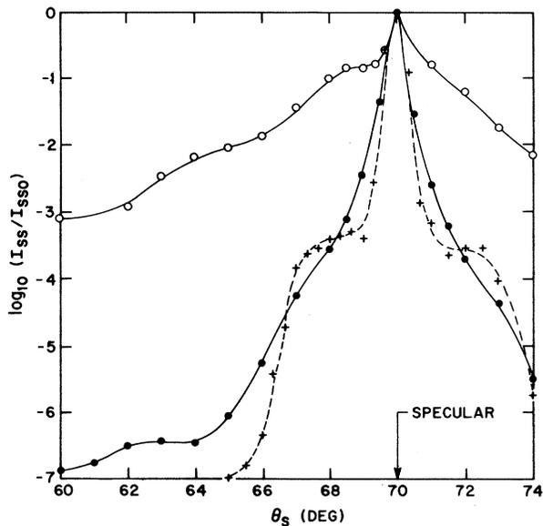
FIG. 1. Scattered light intensity versus observation angle for  $s$ -polarized light ( $A = P = 90^\circ$ ) for Si surfaces: crosses, Syton polished; unfilled circles, NaOH etched; and filled circles, CP-4 etched. Specular reflection occurs at  $70^\circ$ . All data are normalized to the specular intensity.
