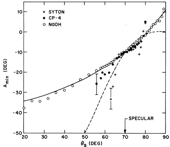
FIG. 2. Analyzer null azimuth versus observation angle for surfaces of Fig. 1 for incident  $70^\circ$  light linearly polarized at  $P = -45^\circ$ . Geometric-optics (solid line) and Rayleigh-Fano (dashed line) model calculations are also shown.
