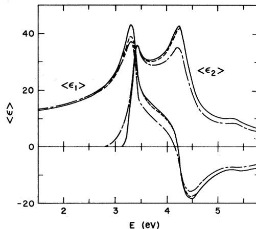
FIG. 3. Pseudo-dielectric-function data  $\langle \epsilon \rangle = \langle \epsilon_1 \rangle + i \langle \epsilon_2 \rangle$  for surfaces of Fig. 1 from specular-component ellipsometry: solid line, Syton and NaOH; long-dashed line, CP-4. Also shown (short-dashed line) is a spectrum obtained by etching a CP-4 surface for 1 min in NaOH.
