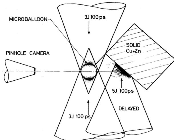
FIG. 1. Experimental configuration for pulsed-x-ray shadowgraphy. The 66- $\mu\text{m}$ -diam microballoon, its support fiber, and the plasma on the brass target are drawn in correct relative scale. The schematic pinhole camera was 2.5 cm from the microballoon.
