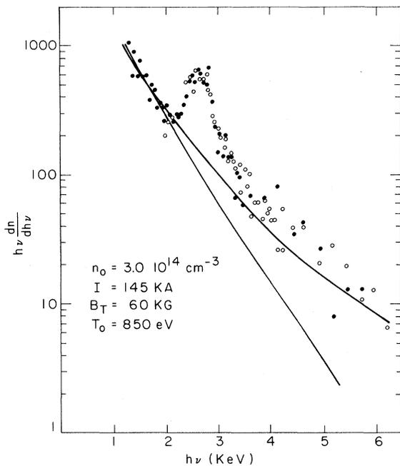
FIG. 1. An x-ray spectrum for a typical nonthermal Alcator discharge. The lower curve is from an 850-eV Maxwellian distribution; the upper curve includes the perturbation induced by magnetic fluctuations.
