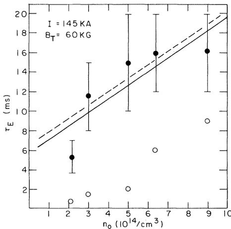
FIG. 2.  $\tau_E$  vs  $\eta_0$ . The open circles are  $\tau_E^*$  deduced from fitting the tail of the x-ray spectrum; uncertainties are about a factor of 2. Solid points are  $\tau_E$  determined from energy content divided by the input power. The dashed line is from Ref. 11. The solid line is the best linear fit to the points.
