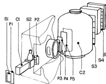
FIG. 1. Perspective drawing of the SLAC Hybrid Facility. The cylindrical bubble chamber is represented in a cut-away drawing of its magnet body. S1 is a scintillation counter. S2–S5 are scintillation hodoscopes. C1 and C2 are Cherenkov counters. P1–P5 are proportional chambers. Steel hadron filters are indicated before S4 and S5.
