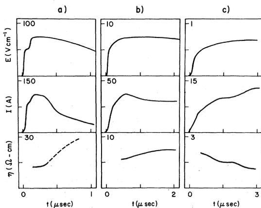
FIG. 1. Representative wave forms for the applied electric field  $E(t)$ , plasma current  $I(t)$ , and inferred resistivity  $\eta(t)$ . Different pulse lengths are obtained by a choice of discharge capacitor and series inductor. Dashed line in (a) indicates that the increasing resistivity is probably due to plasma loss.
