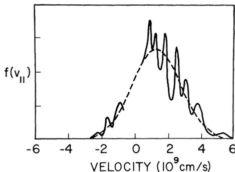
FIG. 4. Typical electron parallel velocity distribution obtained from the  $\vec{E} \times \vec{B}$  particle analyzer. Time  $t = 600\omega_{pe}^{-1} = 75$  ns from application of a step function electric field of 25 V/cm. Dashed line is a Maxwellian of the same  $T_e$  (1200 eV) and  $v_d$ .
