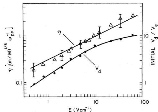
FIG. 2. Average resistivity  $\eta$ , plotted in units of  $(m/M)^{1/3}\omega_{pe}^{-1}$ , as a function of average applied electric field (runaway field  $\sim 10^{-2}$  V/cm). The solid line through the triangles shows a  $\eta \propto E^{1/2}$  fit. Also plotted is the value of  $v_d$  just prior to breakover from free acceleration, normalized to the initial  $v_e \sim 2 \times 10^8$  cm/s;  $n_e \sim 2 \times 10^{10} \text{ cm}^{-3}$ .
