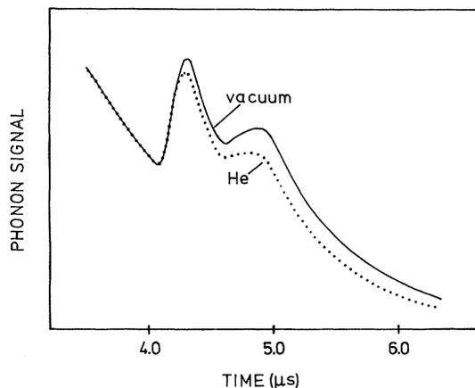
FIG. 3. After the LiF surface of Fig. 1 was exposed to air at room temperature. The helium effect is greatly enhanced.
