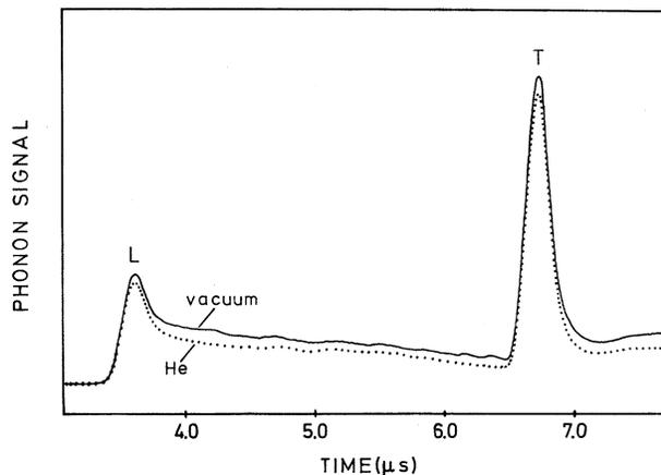
FIG. 2. Longitudinal (L) and transverse (T) echoes from a freshly cleaved NaF surface. The helium effect is not larger on the L phonons than on the T phonons, but is largest for the diffusive tails.
