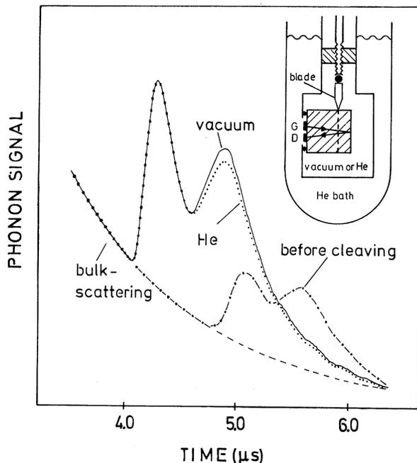
FIG. 1. Phonon pulses reflected from LiF surfaces: dash-dotted line, before cleaving in vacuum; solid line, freshly cleaved at 1 K; dotted line, with helium (the effect is surprisingly small).
