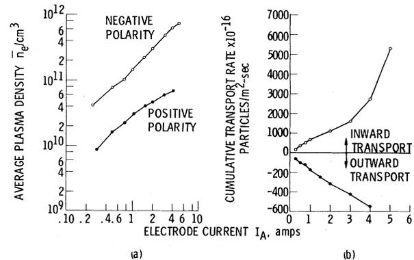
FIG. 2. A paired comparison of the confinement obtained with positive and negative bias of the toroidal plasma for  $B_{max} = 2.4$  T. (a) Average plasma number density as a function of electrode current. (b) Asymptotic cumulative transport rate as a function of electrode current.
