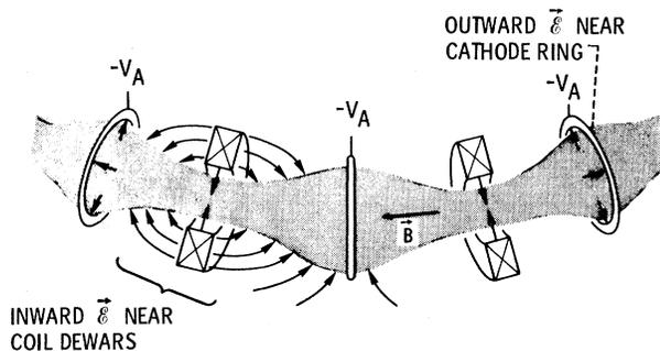
FIG. 1. Schematic of electric field distribution around a negatively biased bumpy-toroidal plasma.
