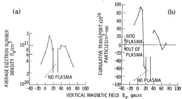
FIG. 4. Effect of a weak vertical magnetic field on plasma containment for negative electrode polarity. (a) Average electron number density as a function of vertical magnetic field. (b) Asymptotic cumulative transport rate at the location of the probe as a function of vertical magnetic field.
