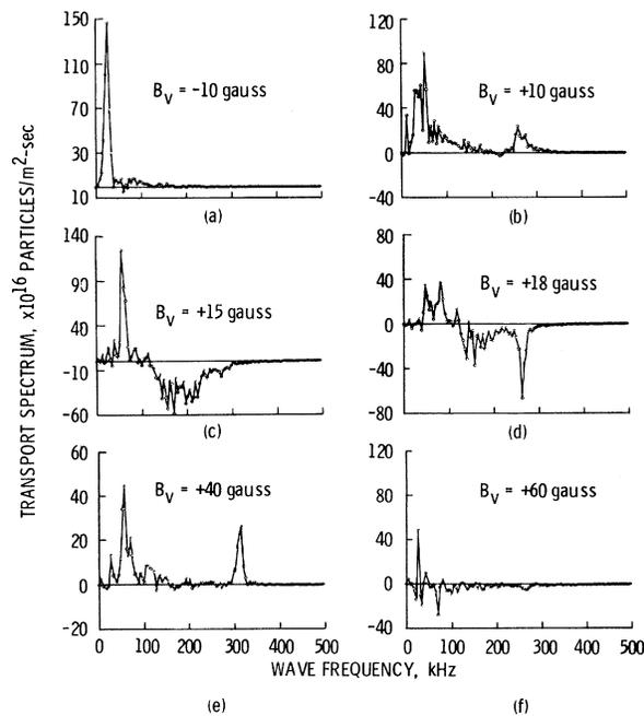
FIG. 5. The transport spectrum as a function of frequency from 0 to 500 kHz. The vertical magnetic field  $B_v$  is equal to (a) -10 G, (b) +10 G, (c) +15 G, (d) +18 G, (e) +40 G, and (f) +60 G.
