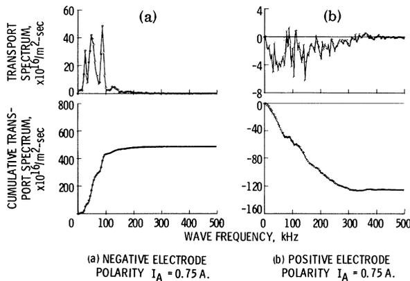
FIG. 3. Transport spectra and asymptotic cumulative transport rates for an electrode current of  $I_a = 0.75$  A. (a) Negative electrode polarity, (b) positive electrode polarity.
