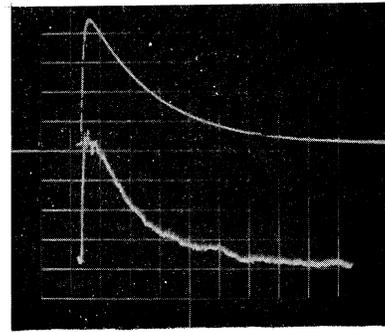
FIG. 2. The upper trace was obtained from a photomultiplier monitoring the  $R$ -line fluorescence ( ${}^2E \rightarrow {}^4A_2$ ) in ruby. The lower trace is a recording of the reflection coefficient of a microwave ruby cavity during the same time interval. The time scale is 2 milliseconds per division. Both recordings followed an intense light pulse which excited the crystal via  ${}^4A_2 \rightarrow {}^4F_2$ .
