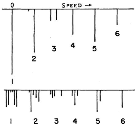
FIG. 1. Theoretical absorption spectra of 14.4-keV resonance radiation from  $\text{Fe}^{57}$ . Top: metallic source and absorber with identical hyperfine splittings. Bottom: same source and absorber but with the splitting in the source increased by 10%.
