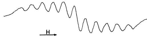
FIG. 1. Hyperfine structure from a nearest neighbor pair of Mn^{2+} ions in the S=1 state. The spacing between adjacent lines is 43 gauss.
