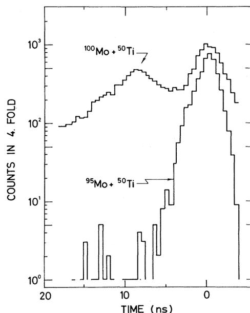
FIG. 2. Time spectra of fourfold events for 230-MeV <sup>50</sup>Ti projectiles on <sup>100</sup>Mo and <sup>95</sup>Mo targets.
