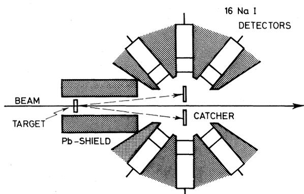
FIG. 1. Schematic diagram of recoil catcher and sixteen-element multiplicity filter apparatus used in search for high-spin isomers.
