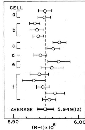
FIG. 2. Summary of pressure-corrected extrapolated data for  $R \equiv g_J(^{87}\text{Rb})/g_S(e)$  at 15°C. The rms error is shown associated with the average.
