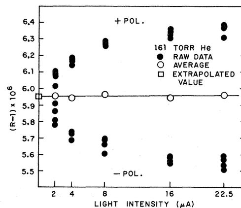
FIG. 1. Extrapolation of the average of  $R$  obtained with the two circular polarizations of light vs light intensity. The least-squares fit to a straight line is shown along with the extrapolated value.
