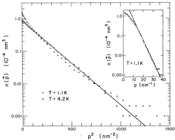
FIG. 1. The momentum distribution in liquid  ${}^4\text{He}$  at  $T=1.1$  and  $4.2$  K as a function of  $p^2$  and (inset) at  $T=1.1$  K as a function of  $p$ . These results were obtained as described in the text from nine scattered-neutron distributions (Ref. 10) in the range  $60 \leq Q \leq 80$   $\text{nm}^{-1}$ .
