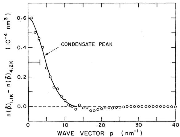
FIG. 2. Temperature change in the momentum distribution in liquid  ${}^4\text{He}$  between 4.2 and 1.1 K. The horizontal line indicates the resolution width.
