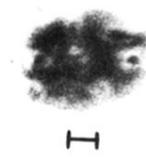
FIG. 3. X-ray micrograph,  $\bar{E}_\nu \approx 2.5$  keV, taken at a  $45^\circ$  angle from the front surface of a W-glass target at  $5.7 \times 10^{14}$  W/cm<sup>2</sup>. The bar denotes 100  $\mu$ m.
