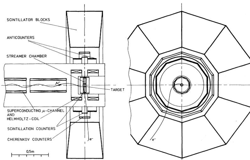
FIG. 1. Lay-out of the  $\mu$ - $e$ -conversion experiment. In both views, there is shown the track of a hypothetical muon-produced 105-MeV electron, bent in a central magnetic field of 3.5 T.
