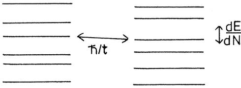
FIG. 1. Energy levels on two adjacent similar blocks of material. The spacing between energy levels is  $dE/dN$  and the coupling between levels in the two blocks is  $\hbar/t$  where  $t$  is given by Eq. (1).
