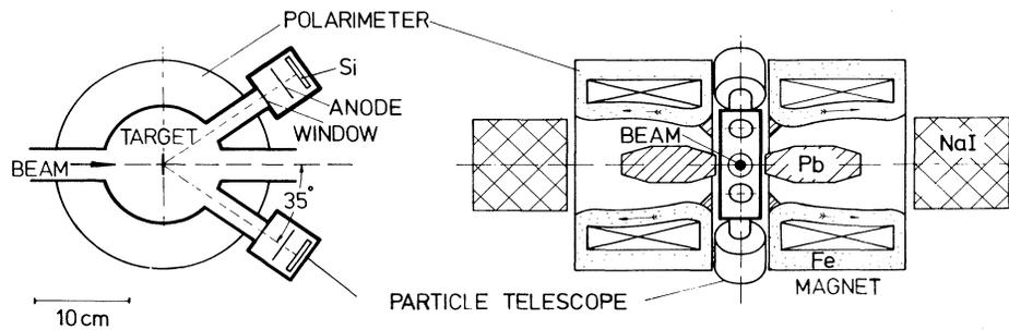
FIG. 1. Detector arrangement. The left-hand side of the figure is a cut of the apparatus along the scattering plane. The right-hand side is a cut containing the scattering normal viewed along the beam direction. The arrows in the magnets indicate the direction of magnetization.
