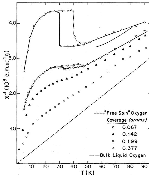
FIG. 2. Inverse susceptibility vs temperature for a series of high coverages. Solid lines are cooling curves and broken lines are warming curves. Pore filling occurs at 0.404 g. Bulk liquid data were obtained in an earlier phase of the present work.
