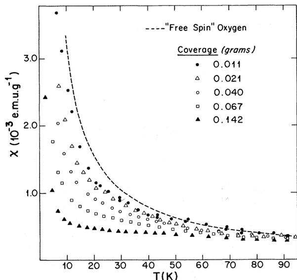
FIG. 1. Susceptibility vs temperature for a series of coverages. (One monolayer corresponds to 0.097 g assuming an oxygen adsorption area of  $12.9 \text{ \AA}^2$  per molecule.) The "free-spin" susceptibility is given by  $\chi = 0.0313 T (\text{K})^{-1} \text{ emu g}^{-1}$ .
