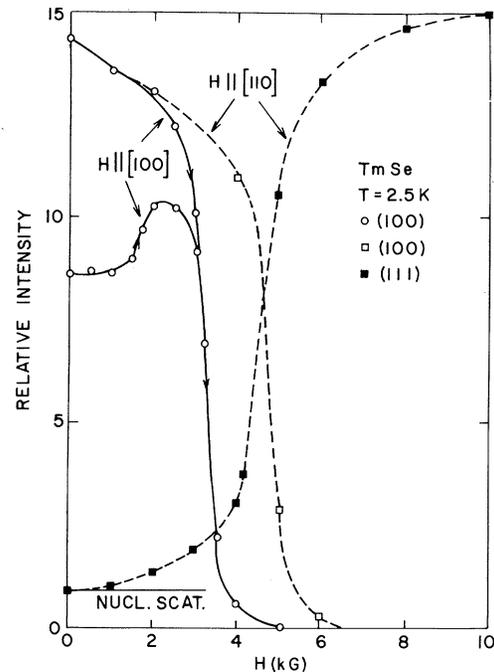
FIG. 2. Relative intensity of Bragg reflections vs applied magnetic field at  $T = 2.75$  K.
