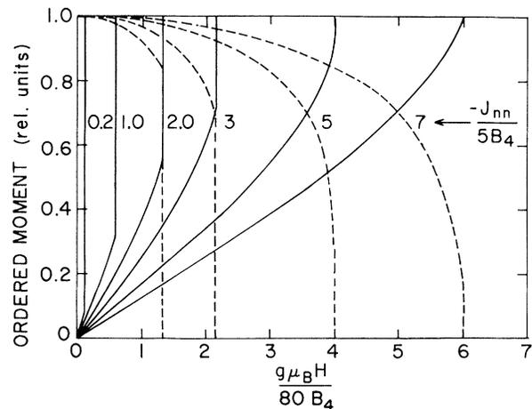
FIG. 3. Theoretical values for the ferromagnetic and antiferromagnetic (shown dashed) moment as a function of  $g\mu_B H/80B_4$  for various values of the reduced exchange  $-J_{nn}/5B_4$ , calculated from Eqs. (2) and (3).
