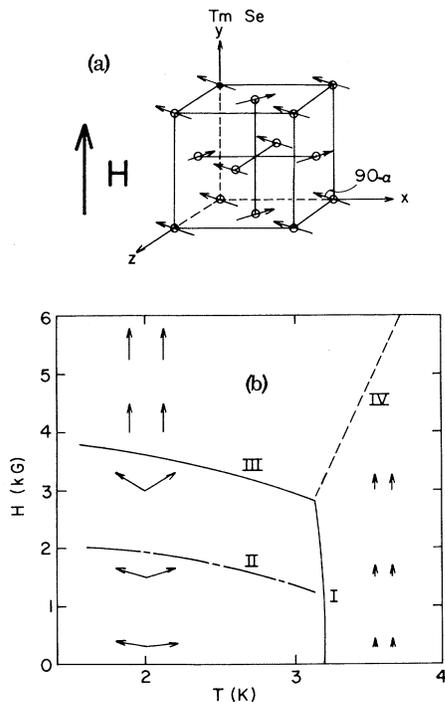
FIG. 1. (a) Magnetic structure of monodomain TmSe for a field along the (010) direction. The tetragonal axis is along the  $z$  direction. A modest magnetic field turns all of the spins through the angle  $\alpha$  out of their positions along (100) in zero field. (b) Magnetic phase diagram of TmSe with the magnetic field applied in the (100) direction.
