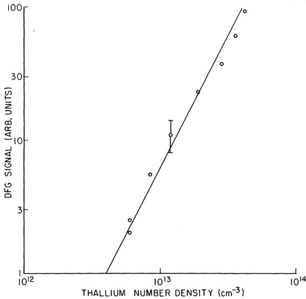
FIG. 1. DFG signal vs. Tl number density  $N$ . Conditions:  $(\omega_1 - \omega_0)/2\pi c = +5 \text{ cm}^{-1}$ ,  $H = 90 \text{ G}$ . Laser linewidths and peak powers:  $0.03 \text{ cm}^{-1}$  and  $\approx 100 \text{ W}$ , respectively. Vertical scale: each unit  $\approx 5 \mu\text{W}$  peak DFG power. The straight line drawn has a slope of 2 on the log-log plot. The error bar represents a typical standard deviation of the signal.
