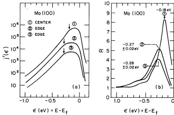
FIG. 1. (a) FEED at the center (curve 1) and two other positions of the (100) plane near its step edge. (Curve 3 is the one nearest to the edge.) (b) The corresponding enhancement factors  $R(\epsilon) = j'(\epsilon)/j'_0(\epsilon)$ , where  $j'(\epsilon)$  is the measured FEED and  $j'_0(\epsilon)$  is the free-electron FEED. The number associated with each arrow indicates the energy position of each peak in the units of eV. Data are taken at 78 K.
