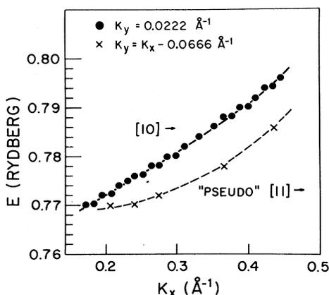
FIG. 3. The dispersion of resonances of Mo(100) as calculated along two directions which are very close to the [10] and [11] directions.
