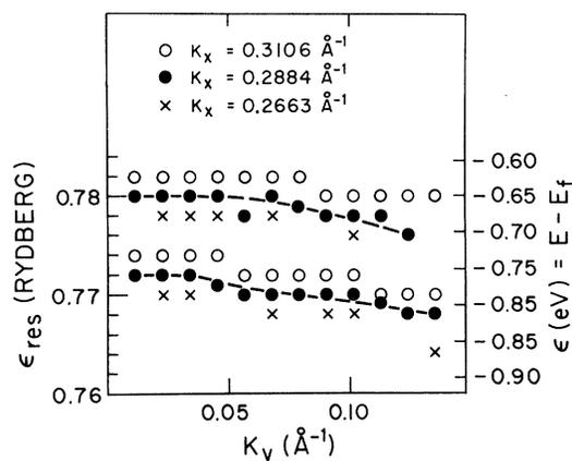
FIG. 4. The dispersion of resonances on Mo(100) as calculated along  $k_y$  for some fixed  $k_x$ .
