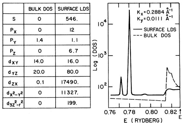
FIG. 5. The calculated SLDS of one major surface resonance (right). The table gives the contribution from all nine bands to the SLDS of this resonance. The densities are in arbitrary units.
