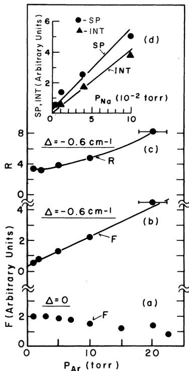
FIG. 3. (a), (b) Dependence of total re-emitted intensity ( $F$ ) on Ar pressure for  $p_{\text{Na}} = 0.1$  Torr and (a)  $\Delta = 0$  and (b)  $\Delta = -0.6 \text{ cm}^{-1}$ . (c) Dependence of  $R$  on  $p_{\text{Ar}}$  for  $p_{\text{Na}} = 0.1$  Torr and  $\Delta = -0.6 \text{ cm}^{-1}$ . (d) Dependence on sodium pressure of the intercept (INT) and of the slope (SP) of  $F$  vs  $p_{\text{Ar}}$  plots.
