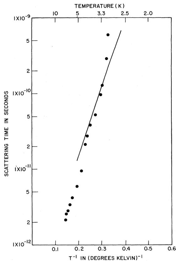
FIG. 3. Experimental quasiparticle scattering time as a function of  $T^{-1}$  (solid circles). The solid line is the theoretical recombination lifetime at  $\Delta(T)$  obtained from Ref. 2.
