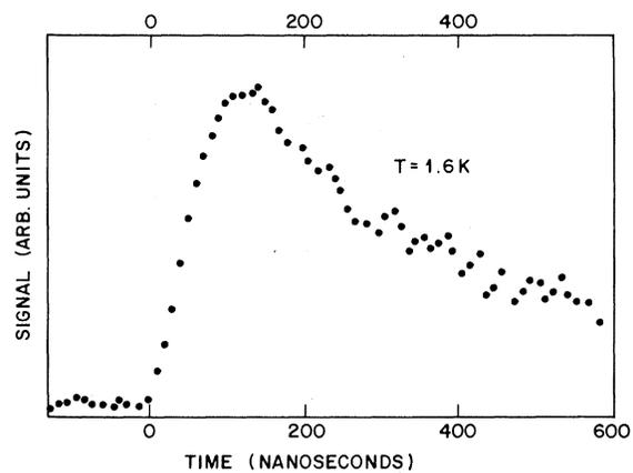
FIG. 2. Expanded trace of the low-temperature (1.6 K) quasiparticle pulse. Propagation length and orientation same as in Fig. 1.
