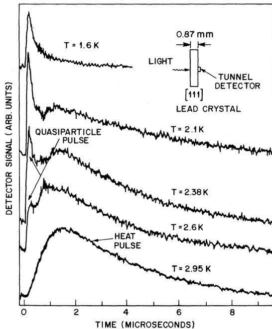
FIG. 1. Tunnel detector signal as a function of time for five different temperatures. Single-crystal lead; propagation length 0.87 mm; orientation [111]. As the temperature is lowered below about 2.6 K one observes the decoupling of the quasiparticles from the heat pulse. See text.
