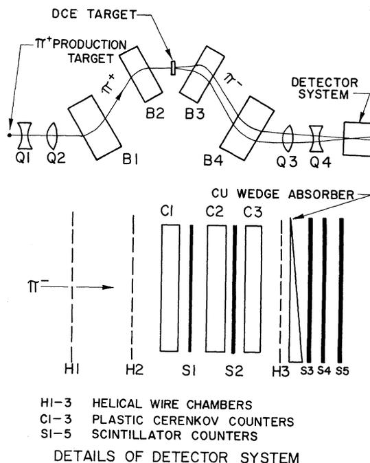
FIG. 1. Schematic layout of the LAMPF low-energy pion channel and DCE spectrometer.
