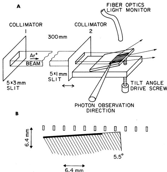
FIG. 1. (a) shows the experimental arrangement. (b) indicates the positioning of the surface relative to the rectangular observation areas ( $0.2 \times 1.5$  mm<sup>2</sup>) from which light was observed. A series of positions along the beam is shown at a fixed height above the surface. The height was also adjustable.
