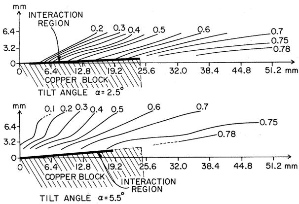
FIG. 3. Contours of equal circular polarization  $S/I$  for Ar II, 4610 Å for copper surface tilt angles of  $2.5^\circ$  and  $5.5^\circ$ .
