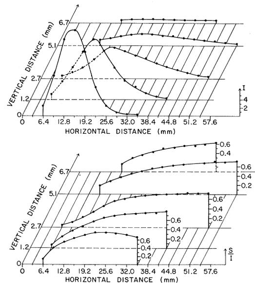
FIG. 2. Total intensity (top), and circular polarization fraction  $S/I$  (bottom) of Ar II 4610 Å shown as two-dimensional functions of the horizontal distance along the beam and the vertical distance above the surface. The interaction region is located between 0 and 19.2 mm, is tilted at  $5.5^\circ$  to the horizontal and its top-most point is near zero in the vertical direction.
