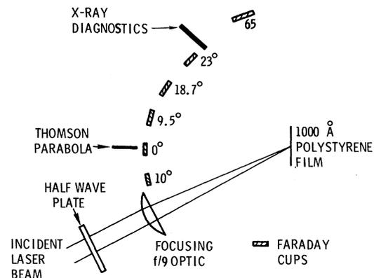
FIG. 1. Experimental configuration for study of polarization dependence.
