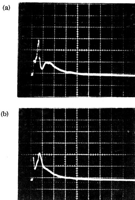
FIG. 2. (a) Upper: Time history of Faraday-cup current for  $p$ -polarized laser irradiation. (b) Lower: Time history of Faraday-cup current for  $s$ -polarized laser irradiation.
