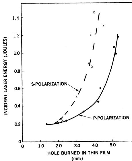
FIG. 3. Diameter of hole burned in thin-film target as a function of incident laser energy for a 50-ps full width at half-maximum laser pulse.
