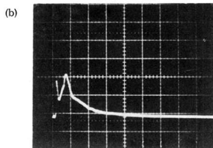
FIG. 2. (a) Upper: Time history of Faraday-cup current for  $p$ -polarized laser irradiation. (b) Lower: Time history of Faraday-cup current for  $s$ -polarized laser irradiation.
