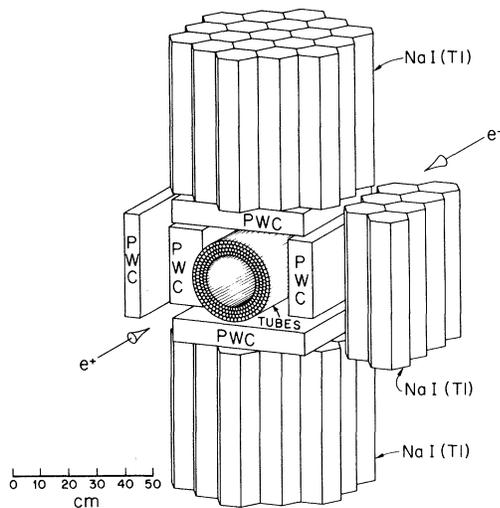
FIG. 1. Schematic of the apparatus used for the inclusive  $\gamma$ -ray experiment. The tube counters provide azimuthal coordinates for charged-particle trajectories, while the proportional wire chambers (PWC) yield coordinates along the beam direction. The hexagonal NaI(Tl) modules are 20 radiation lengths thick.
