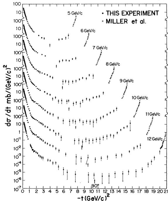
FIG. 2. Neutron-proton differential cross sections. The  $\uparrow$  indicates the position of  $90^\circ$  in the c.m. systems.
