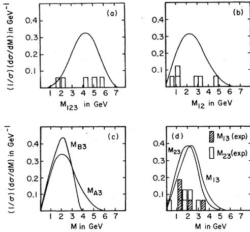
FIG. 2. (a) The trimuon invariant-mass spectrum. We give the experimental values as boxes. (For errors see Ref. 1.) (b)–(d) Spectra in the invariant masses of the muon pairs. The effect of ordering the momenta is to convert (c) into (d).
