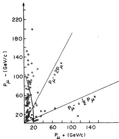
FIG. 1. Positive- and negative-muon momentum scatter plot for dimuon recorded in the previous Harvard-Pennsylvania-Wisconsin-Fermilab experiments that used a quadrupole-triplet or bare-target neutrino beam. The solid line indicates the results of a Monte Carlo calculation for charmed-particle production by Barger and Gottschalk (Ref. 6). No events were generated outside the solid line from a sample of 1000 dimuons.
