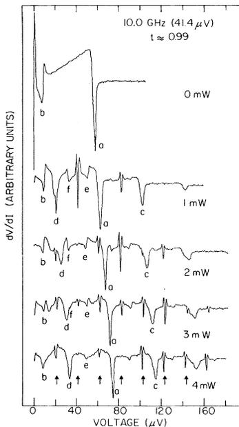
FIG. 1.  $dV/dI$  vs voltage for Al- $\text{Al}_2\text{O}_3$ -Al tunnel junction on  $\text{BaF}_2$  substrate.
