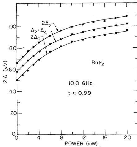
FIG. 2.  $2\Delta_>$ ,  $\Delta_> + \Delta_<$ , and  $2\Delta_<$  vs microwave power for Al-Al<sub>2</sub>O<sub>3</sub>-Al junction.
