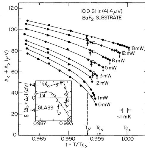
FIG. 3.  $\Delta_< + \Delta_>$  vs reduced temperature at several levels of microwave power for Al-Al<sub>2</sub>O<sub>3</sub>-Al junction on BaF<sub>2</sub> substrate. Inset shows gap enhancement,  $\delta(\Delta_> + \Delta_<)$ , vs temperature for Al-Al<sub>2</sub>O<sub>3</sub>-Al junction on a glass substrate at (a) 9.9 GHz and (b) 11.9 GHz. The appropriate values of  $T_{\nu}$  are indicated.
