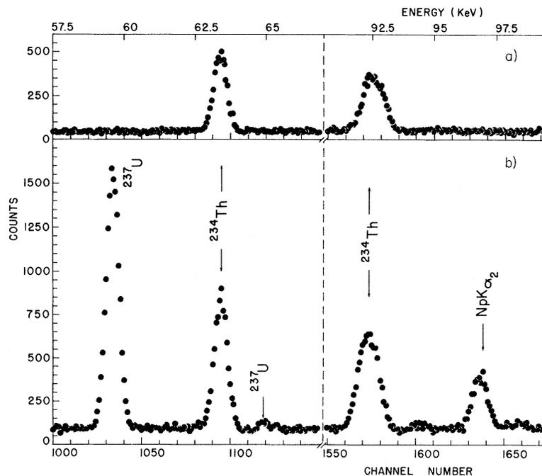
FIG. 2. Typical pulse-height spectrum: (a) prior to bombardment; (b) after bombardment.
