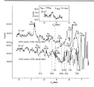
FIG. 1. 12° and 33° spectra from the reaction  $^{208}$ Pb(p, p') at 45 MeV. The contaminant peaks are blackened and the L = 0 and L = 1 peaks are cross hatched. A typical background used to determine the intensity is indicated for two of the peaks. The inset shows part of a 10° spectrum from the reaction  $^{208}$ Pb(<sup>3</sup>He, <sup>3</sup>He') at 70 MeV.
