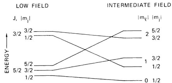
FIG. 2. Correlation diagram between low and intermediate field showing the connection between the low-field  $|m_j|$  states and the intermediate-field  $|m_l|$  states.
