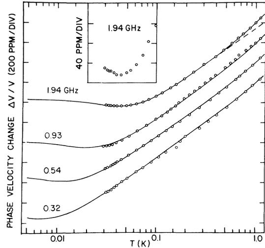
FIG. 1. Relative phase velocity of longitudinal sound waves in Suprasil fused silica glass as a function of frequency and temperature. The dashed line shows the phase velocity expected from the two-level model with a constant density of states; the solid line shows the calculated velocity with a quadratic (in energy) correction term added to  $\bar{n}(\epsilon)$ . Each frequency is offset by 200 ppm at 1 K. The inset shows the region near the velocity minimum.
