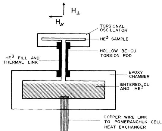
FIG. 1. Schematic of the apparatus. The drive and detector electrodes are not shown. The  $^3\text{He}$  and  $^{195}\text{Pt}$  NMR coils have also been omitted.
