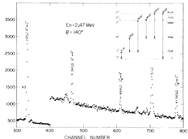
FIG. 3.  $(n, n'\gamma)$  photon spectra for the rotational nucleus  $^{152}\text{Sm}$ . The peaks in the spectrum can be identified with rotational and vibrational transitions in the level scheme shown.
