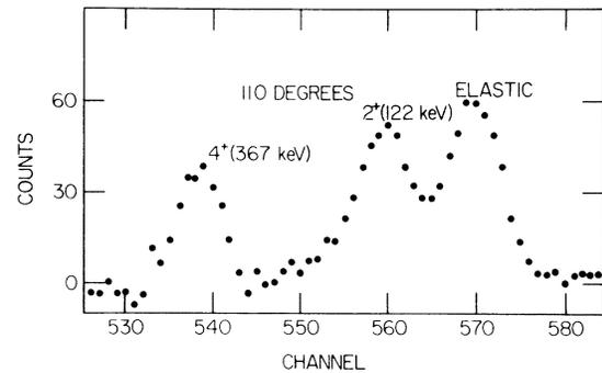
FIG. 2.  $^{152}\text{Sm} + n$  time-of-flight spectrum for 2.47-MeV incident neutrons. Background contributions are subtracted. The three peaks are identified with the elastic scattering and scattering from the first two excited levels of  $^{152}\text{Sm}$ .
