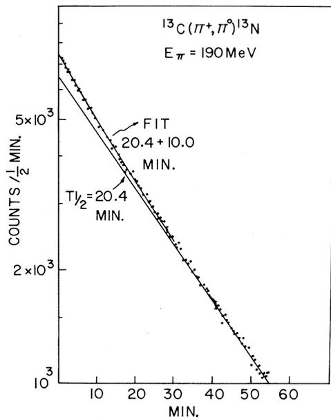
FIG. 2.  $\beta^+$  decay curve, measured by the coincident detection of the annihilation  $\gamma$  rays. The fit has a normalized  $\chi^2$  value of 1.1. The lower solid line shows the contribution of the 20.4-min  $\beta^+$  activity of  $^{11}\text{C}$ . The rest is the 10-min  $^{13}\text{N}$  activity.
