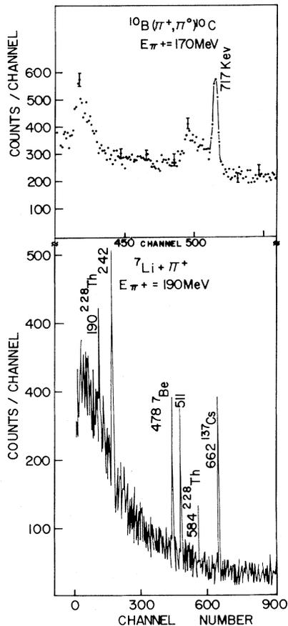
FIG. 1.  $\gamma$  spectra from targets of <sup>7</sup>Li and <sup>10</sup>B. The  $\gamma$  radioactivity from the <sup>7</sup>Li target was counted for 30 h, 120 days after the irradiation; the 478-keV line comes from the <sup>7</sup>Be activity. The radioactivity from the <sup>10</sup>B target was counted while the target was mounted on a physical pendulum. The 717-keV line comes from <sup>10</sup>C activity.
