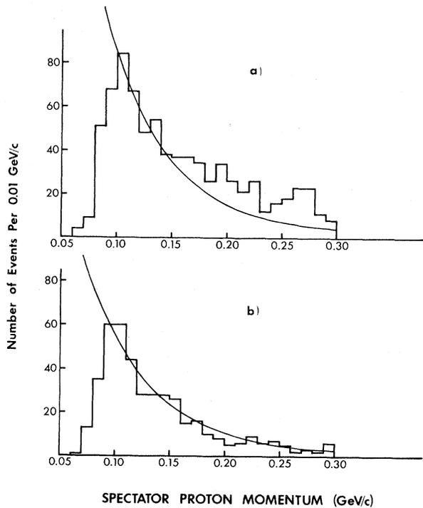
FIG. 3. Spectator-proton momentum distributions for all neutronlike events with visible spectator proton for (a) events with spectator in the forward hemisphere and (b) events with spectator in the backward hemisphere. The solid curves show the predictions of the Hulthén wave function (Ref.4) normalized to the number of events with spectator momenta between 0.10 and 0.15 GeV/c. The events are not weighted for geometrical losses; these corrections do not change the shapes of the distributions.
