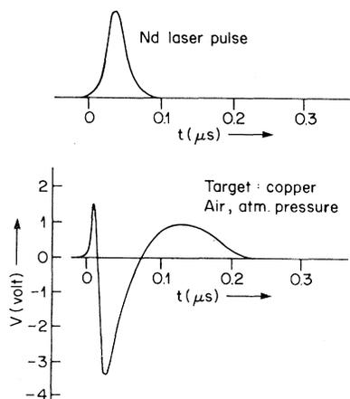
FIG. 2. Typical voltage pulse  $V$  corresponding to the probe  $dI/dt$ .
