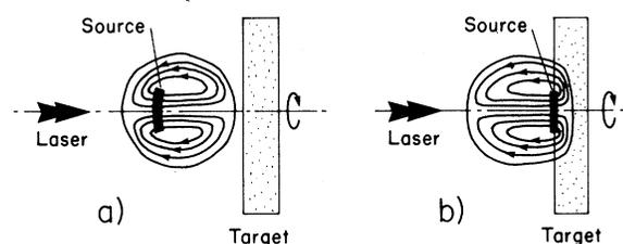
FIG. 4. Two different locations for the current flow paths. The sources are located (a) at the front of the expanding plasma or (b) at the plasma-target interface.
