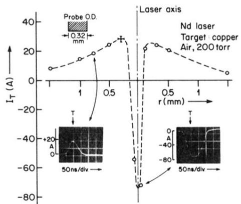
FIG. 3. Typical probe current distribution. A positive value implies conventional current flow across the target surface into the plasma.
